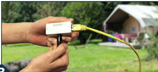
2 Connect one end of the Ethernet cable (not supplied) to the LAN (PoE) port on the EZ Hotspot Extender. The LAN (PoE) port can be founded on the right-hand side as seen from the back of the device.
